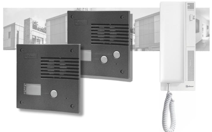
K-201GRF & K-202GRF flush mounting audio kits with vandal resistant (IK-09) and weatherproof (IP-44) door panel. The door panel is 2.5mm thick injected aluminium and in a graphite colour with an attractive curved front. The system has an electronic call to the handsets with an acoustic acknowledgment signal at the door panel.
